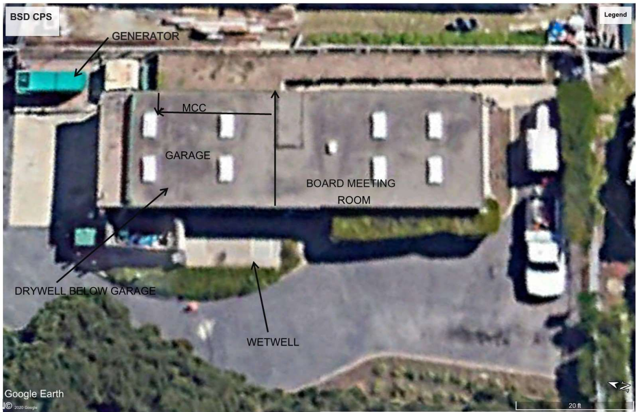
BSD OFFICE AND PUMP STATION LAYOUT
